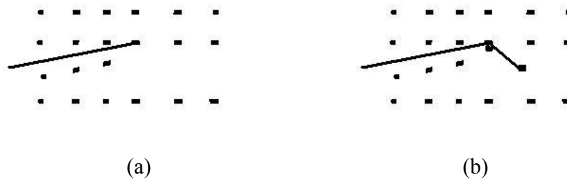
Figure 2.16 Crack propagating using meshless methods where dots represent nodes. (a) The initial configuration; (b) After the crack has grown.
